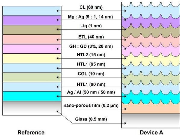
**Figure 3.** Schematic device structure comparison.
