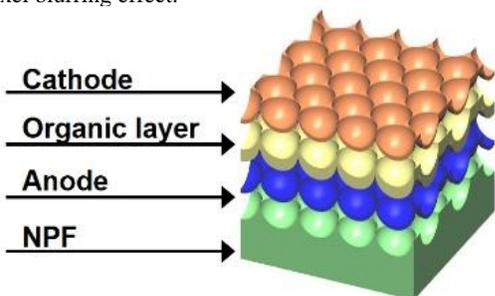
Figure 1. Schematic diagram of TEOLED having concave patterned anode.
